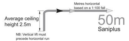
Note: If you increase 'horizontal' pipe fall to full 1:40 gravity fall, then the horizontal distance can be increased to virtually any distance required (also increase pipe size)
