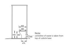
Notes: Dimensions are for doors fully open. Internal dimensions: The width is measured from acrylic panel to acrylic panel. The depth is taken from the back acrylic panel to the inner face of the door.
