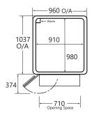
Notes: Dimensions are for doors fully open. **Internal dimensions:** The width is measured from acrylic panel to acrylic panel. The depth is taken from the back acrylic panel to the inner face of the door.
